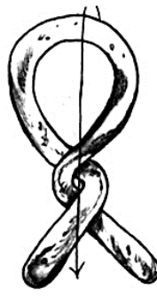
The ends have been crossed twice; now fold the large top loop down, so that it lands on the ends
